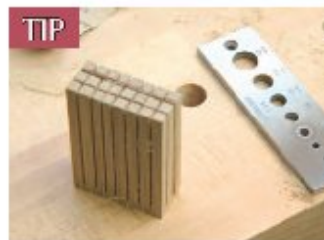
TIP Pegs Paul makes his own dowel for pegging joints by cutting a block of blanks on a bandsaw then using a dowel plate (above)
