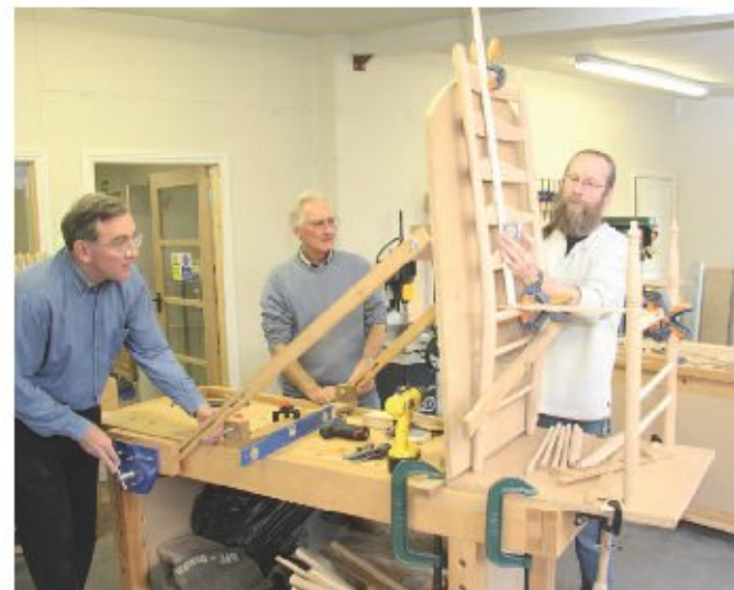
Assembly John Dunlop and Paul Hodgson (top) assembling John's first chair, having marked out the rail holes with Paul's measuring device, which holds the back frame at the right angle
