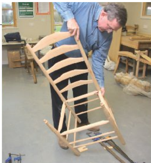
Tolerance Peter Sefton likes his students to try chairmaking because it changes their perspective of tolerances. Paul Hodgson uses a jig to align the front and back frames (left), but John Dunlop has to rely on brawn to straighten up an assembled chair (above)
