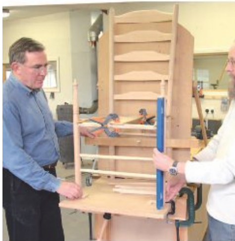
Tolerance Peter Sefton likes his students to try chairmaking because it changes their perspective of tolerances. Paul Hodgson uses a jig to align the front and back frames (left), but John Dunlop has to rely on brawn to straighten up an assembled chair (above)
