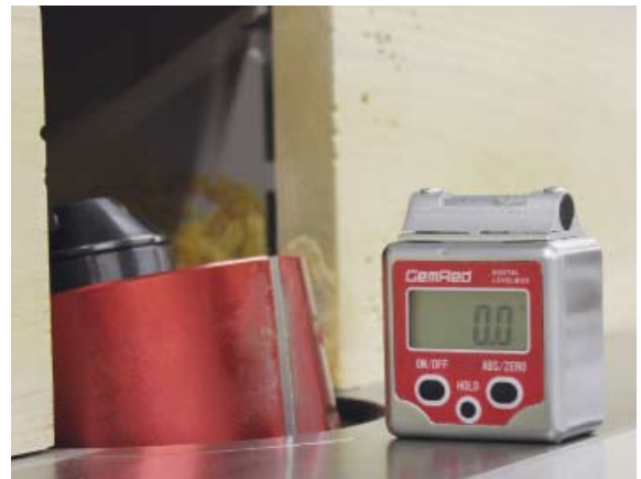
Digital angle gauge on spindle moulder bed
