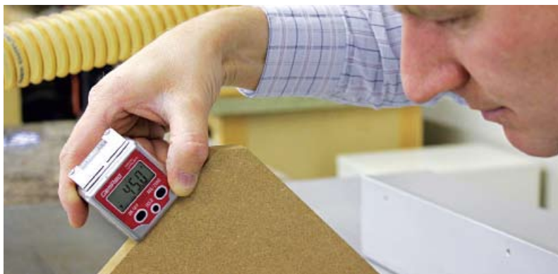
Digital angle gauge on table saw bed
