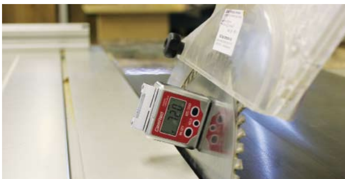
Digital angle gauge attached to canted table saw blade
