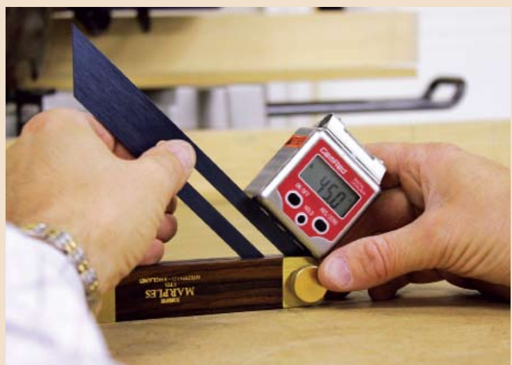
Peter taking an angle reading on the sliding bevel blade
