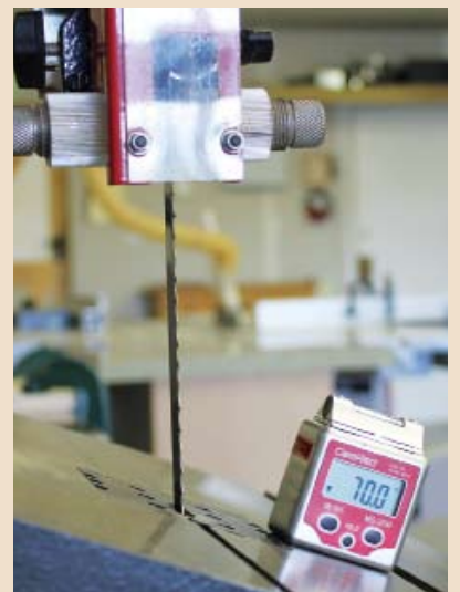
Digital angle gauge to canted bandsaw bed
