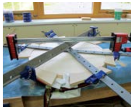
Gluing up the drum sides to the base and top using the MDF offcuts kept from the earlier jig making process. Always keep them as they will come in useful
