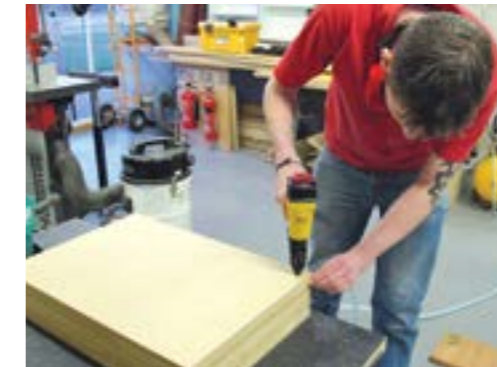
Using a pin gun after applying Titebond glue with the gravity feed roller
