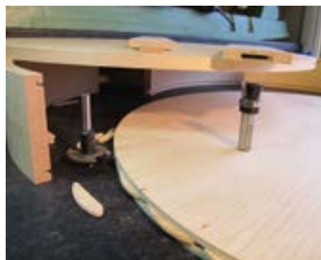
The carcass sides and base have been routed using a 4mm slotting cutter to accept biscuits. The dickie bow-shaped drawer runner is routed and glued in place whilst the drawer muntin is routed and cleaned to run the drawer square into the round carcass
