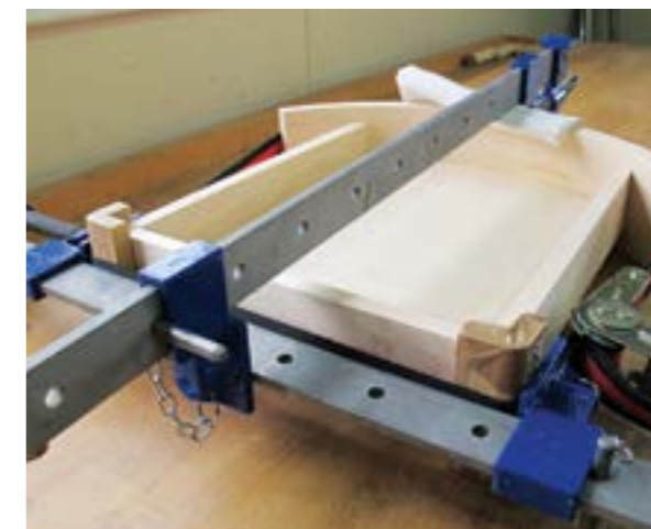
A band cramp and corner blocks pulls the drawer together whilst the sash cramps stops the drawer front from bowing out from the pressure of the band cramps' pull
