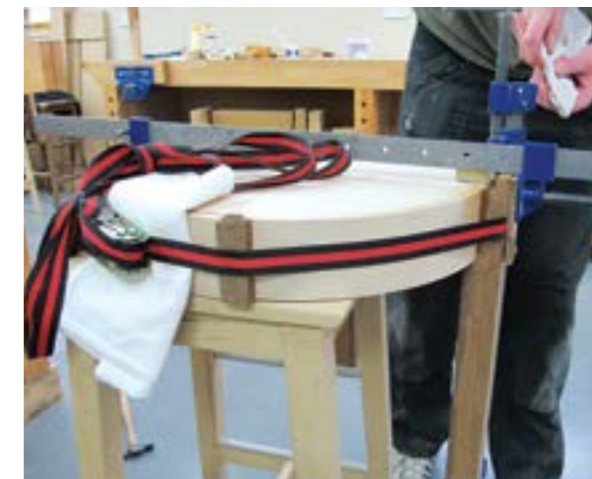
With the drawer in position, the legs and teak mouldings are glued on using the trusty band and sash cramps
