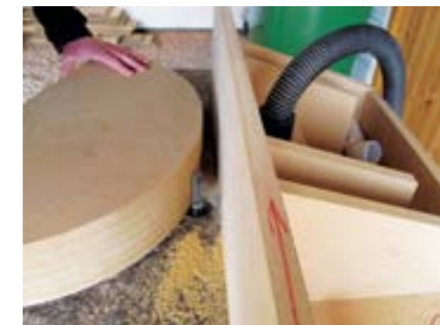
Paul is ousted to the outside when routing off the bandsaw MDF, using a template trim router cutter
