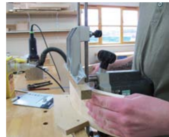
The router has a pair of fences with a round section screwed to the bottom one, to hold and guide the drawer front as the stopped groove is cut for the drawer bottom
