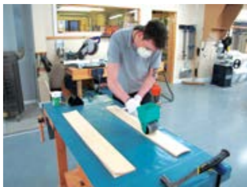
Paul uses the gravity feed roller to apply urea formaldehyde to the constructional veneer to make the drum sides
