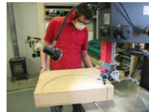
Cutting through male and female formers on the bandsaw after the 15mm groove was made with the router on a tramrel
