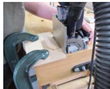
The Domino was used to make the joints between the drawer fronts and sides, using the vice and bench top as a tangent
