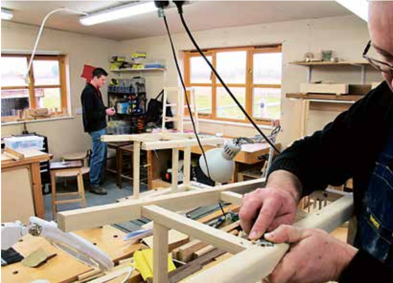
Garry flushing down his walnut dowels, pinning the tenons
