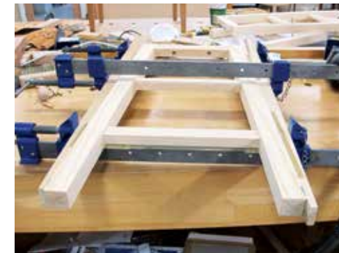
Gluing up the side frame with tapered glue blocks using three cramps to stop the legs twisting
