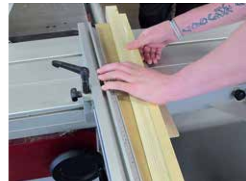
Cutting legs to length on the tablesaw with compound angles
