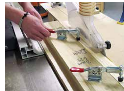
Pushing the taper jig through the saw with legs secured with toggle clamps
