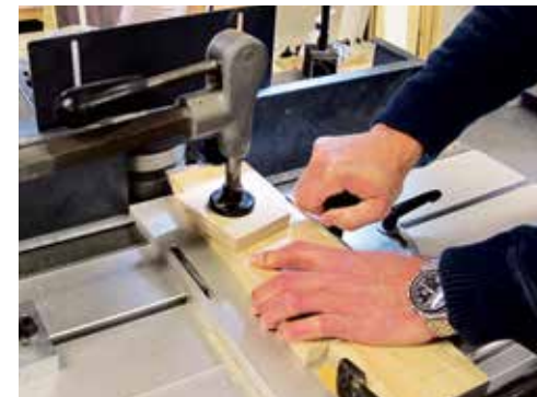
Tenoning on the spindle moulder gives clean and repeatable sloping shoulders
