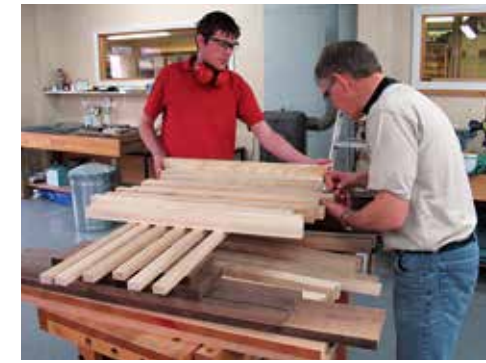
Students Paul and Harry selecting previously machined ash ( Fraxinus excelsior ) to match grain and colour
