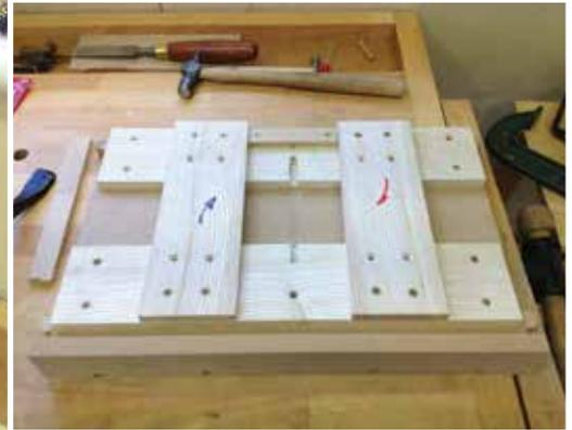
**Main image:** The jig guiding the router base for accuracy
