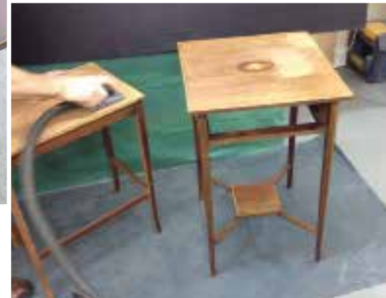
Top: The underside of the Pembroke table in the process of being stripped Above: Cleaning up with abranet, prior to polishing
