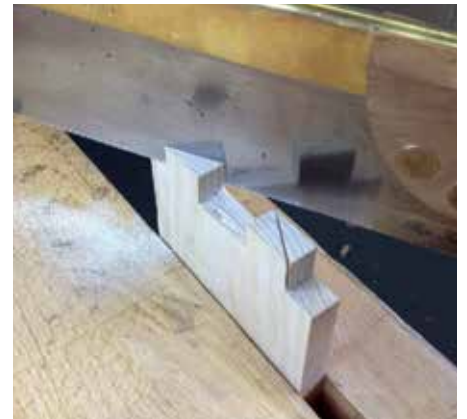
The saw kerf must go exactly corner to corner
