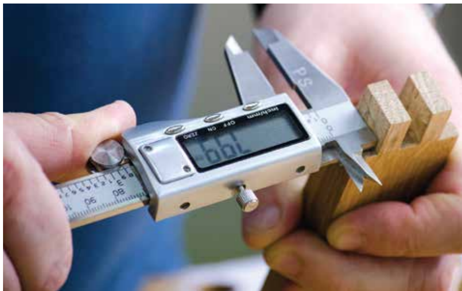
A GemRed digital Vernier calliper checking thickness
