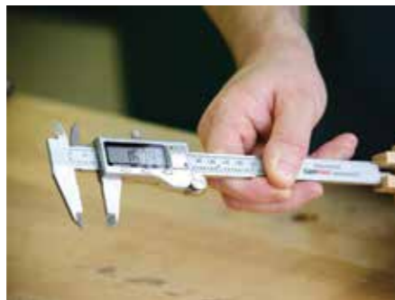
A GemRed digital Vernier calliper checking depth
