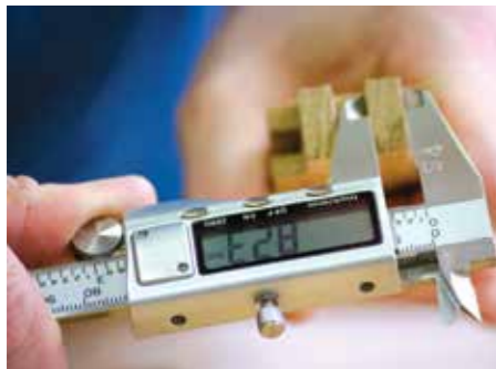
A GemRed digital Vernier calliper checking thickness
