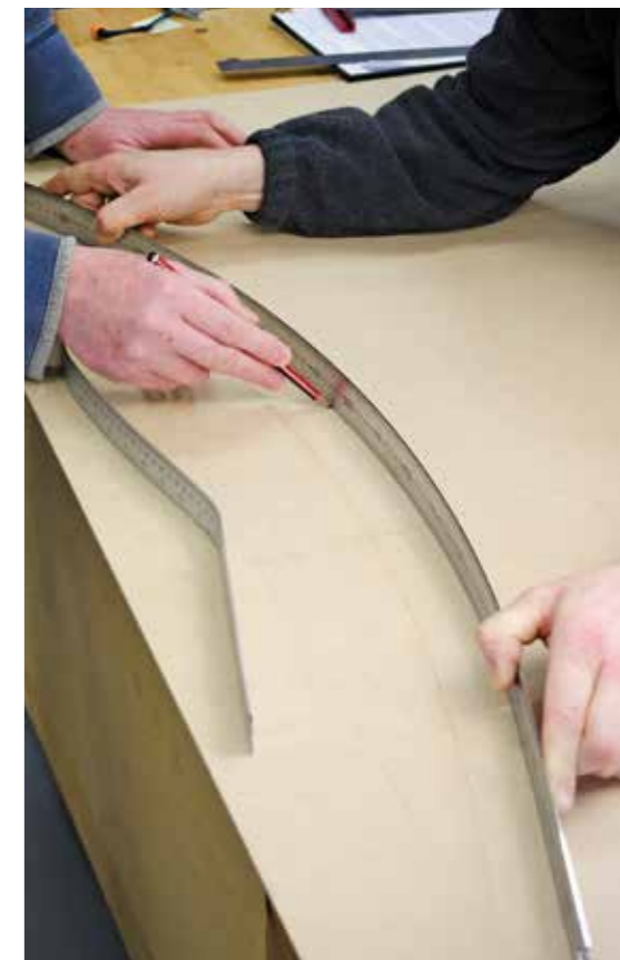
Bending a rule and a bent rule
