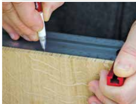
Using an INCRA T-rule for progressive markings
