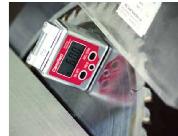
Below: A GemRed bevel box measuring a saw blade
