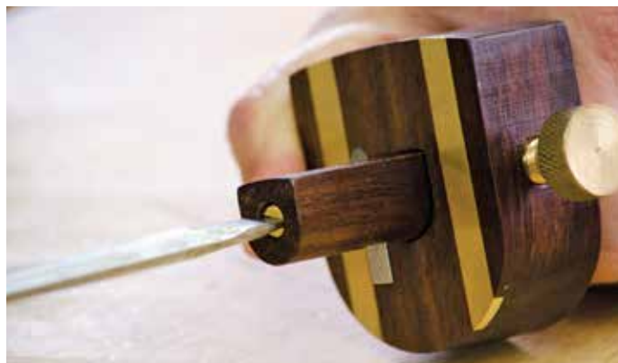
A screw in the end of the stem makes for accurate repositioning
