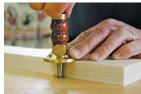
The WoodRiver gauge has a thicker stem and doesn't roll off the bench
