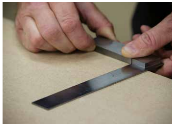
Checking for accuracy using a piece of MDF. Simply lay the square on it with the stock to the left-hand side and scribe a line
