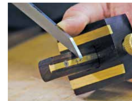
Right: Modifying a mortise gauge by filing the ends and shortening the stem
