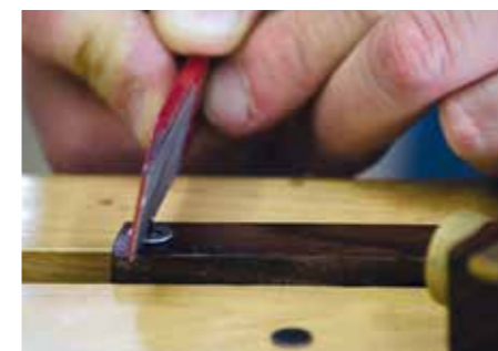
For setting, a ruler is used to set the point of the pin at a desired distance from the gauge's stock or fence
