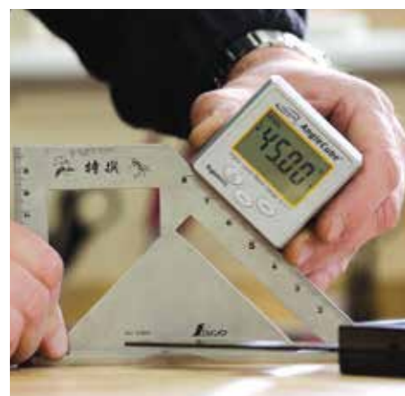
Using my Angle Cube to check 45° squares, which makes it much easier
