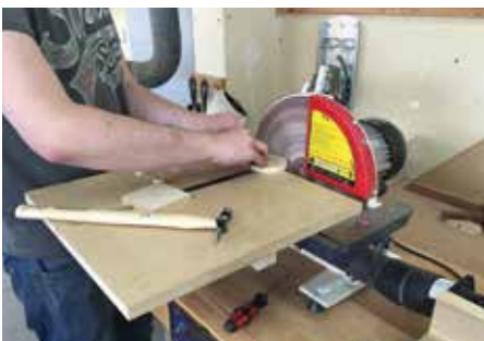
Disc sanding to the required diameter
