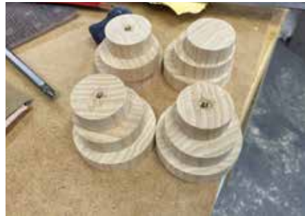
Threaded inserts to form centre fixings
