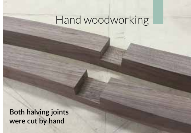
The legs were set up on the rod board and the joints marked out
