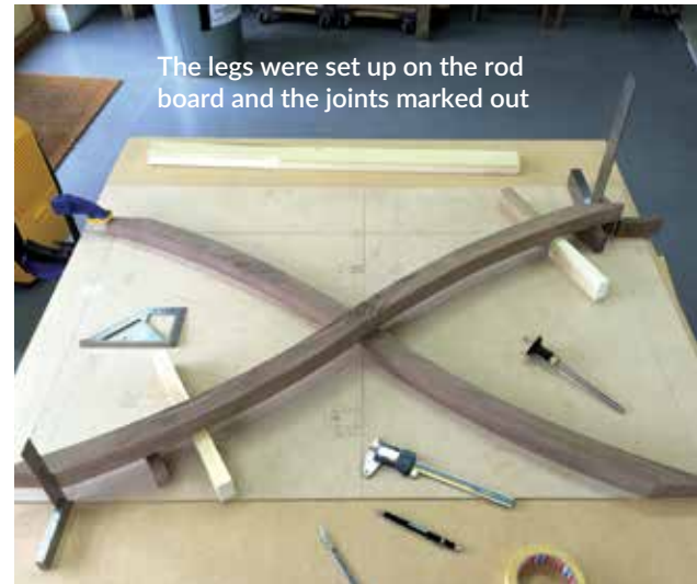
Both halving joints were cut by hand
