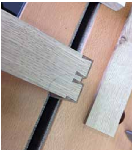
Hounds tooth dovetails to accommodate the central groove for the drawer pull
