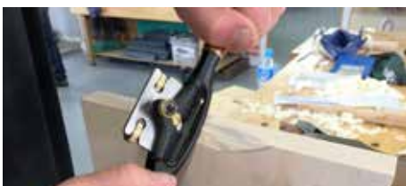
PIC 6. Spokeshaving out carving gouge marks
