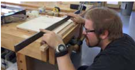
PIC 3. Checking flatness with a Veritas straightedge
