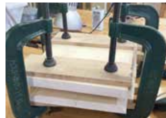
PIC 4. After initial planing the boards are cramped to keep them flat
