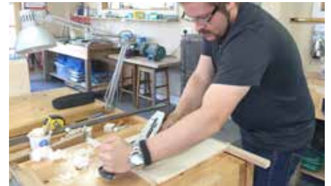
PIC 2. Jack planing to flatten the board
