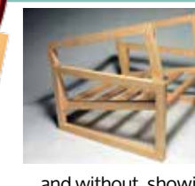
... and without, showing the simple but effective box frame construction
