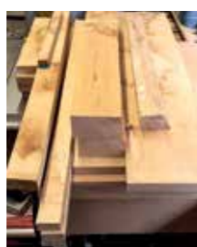
Timber in its raw form, cut oversize and ready for planing
