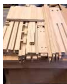
Pieces jointed and cut to size, ready for gluing up
