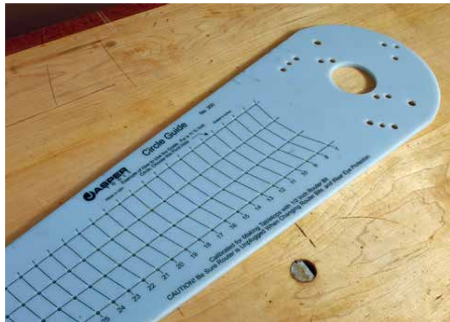
This versatile circle cutting jig is pre-drilled with 6mm increments
