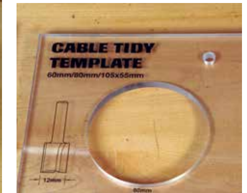
Manufactured jigs come in basic forms but will often require the use of specific cutters and guidebushes
