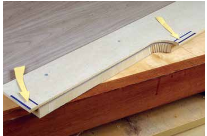
Make your jig longer at both ends of the workpiece for clean entry and exit points
