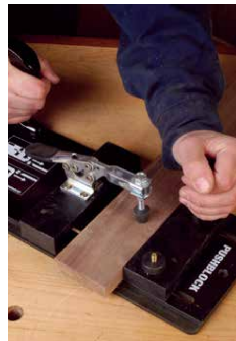
This cross-cutting jig is made from Tufnol and is guided by the fence on a router table
