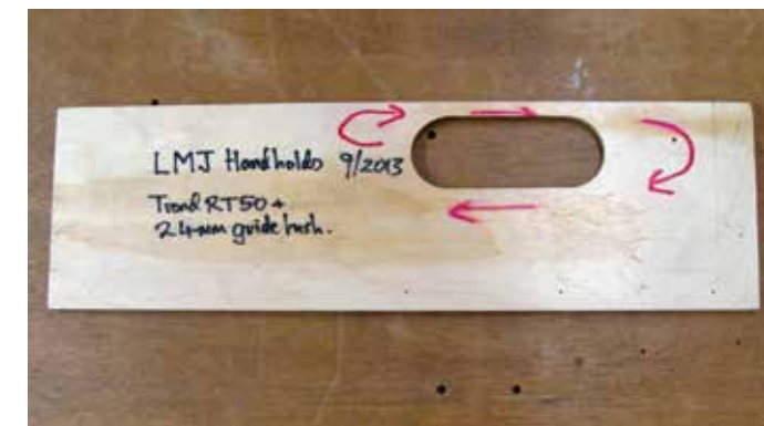
A much-used, but very simple, hand-held cutting jig. While it is very simple, it can be used to make hand-holds of varying sizes by changing the cutter or guidebush
