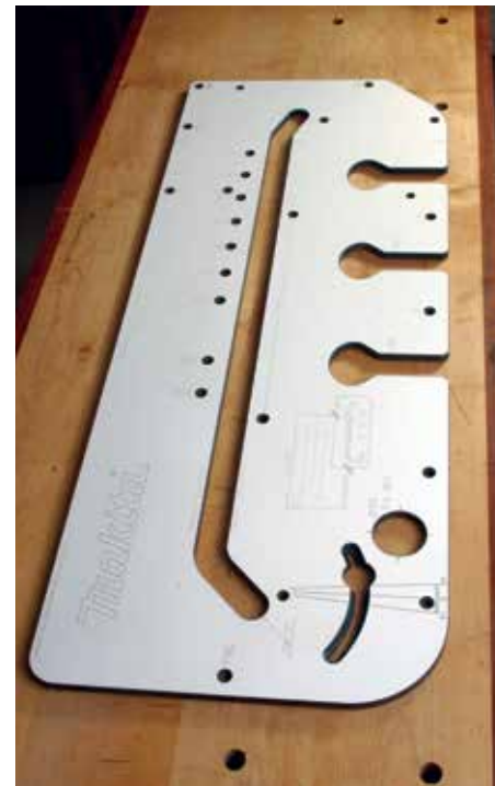
A typical kitchen worktop jig made from hard wearing solid laminate has all the profiles necessary for jointing the ends of worktops
