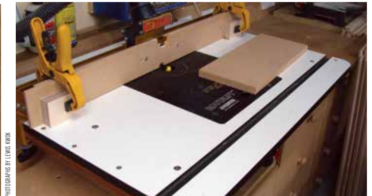
Jigs can be really simple, such as these blocks clamped to a router table fence to achieve a stopped groove
