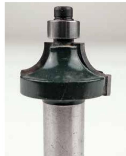
A gap between the bottom of the cutter and the top edge of the bottom-mounted bearing can make a perfect semicircular profile impossible to achieve
