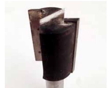
Use a cutter with plunge cutting capability if working into a sacrificial board
