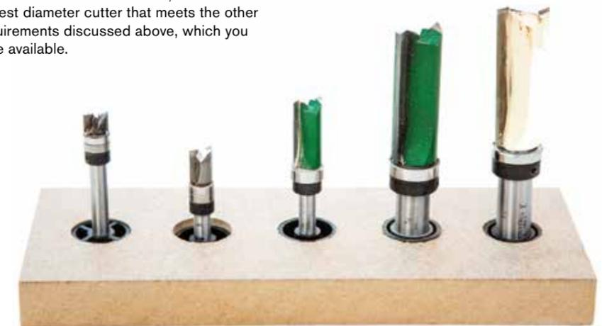
Top-bearing mounted cutters. Straight cutters in various sizes, including two down-shear cutters, from Trend, Axcalibur, Titman, CMT & Wealden on 1/4in, 8mm and 1/2in shanks
