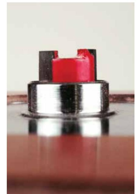
The off-set between the edge of the cutter and guide bush needs to be taken into account
