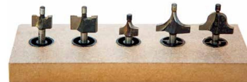
Piloted cutters – a selection of cutters with bottom-mounted pilots
