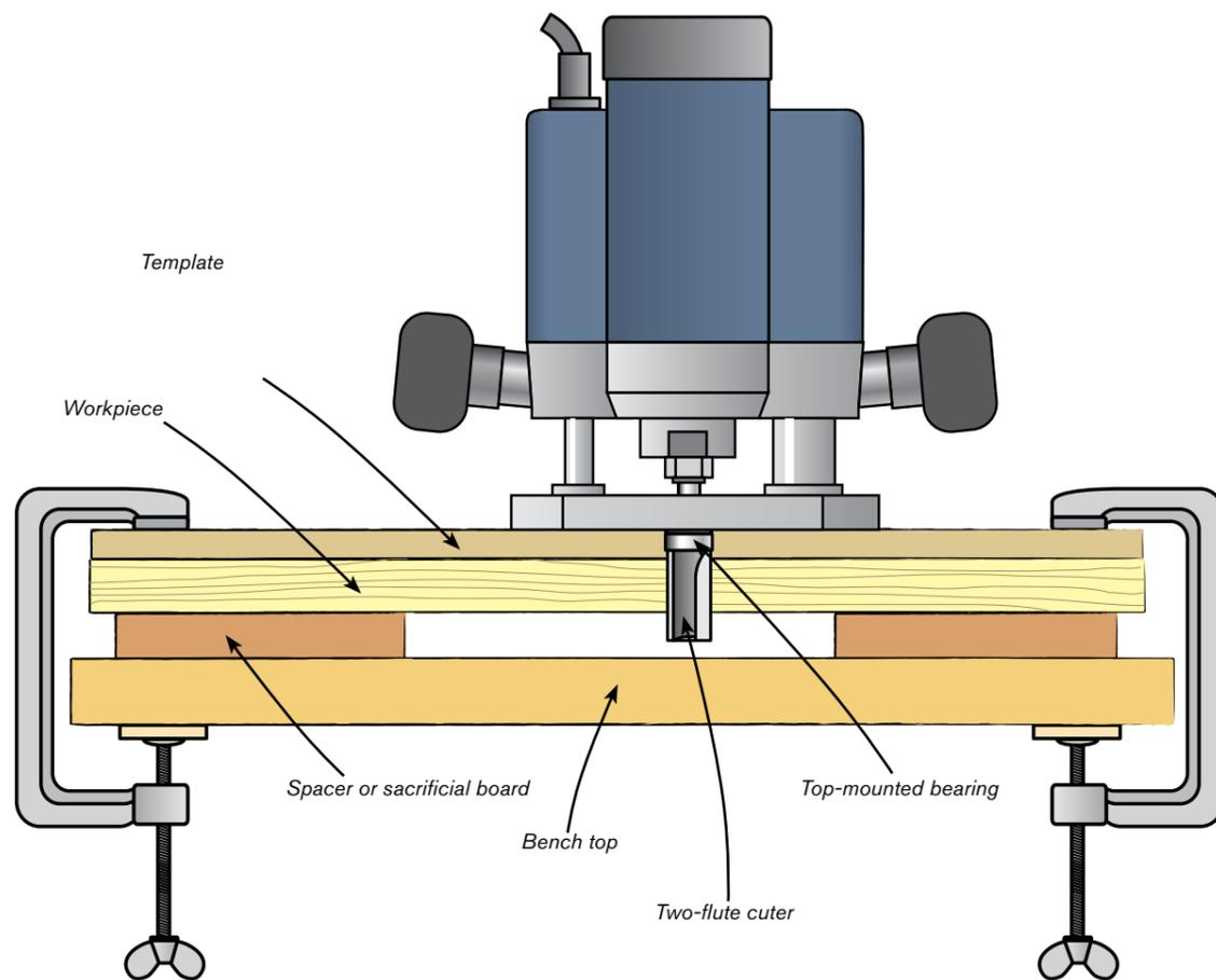
The diagram on this page illustrates a typical setup with a template mounted above the workpiece and using a top-mounted bearing-guided cutter in a hand-held router. It shows clearly the need for spacer blocks to keep the bottom of the router cutter above the workbench. The cutter shown is actually a standard straight cutter, but other variants can be used in the same setup. For example, a down-cut shear or spiral cutter could be used to give a smoother finish on the routed
